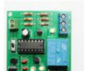
Infrared (IR) remote operated switch by buildcircuit
